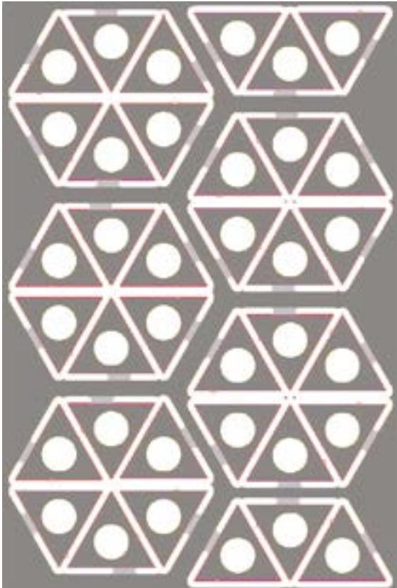
Pocketing: the tool removes all material inside an outline, to a specified depth. Pocketing tool paths only work within **closed** shapes, all lines must be **joined without any overlaps**.
